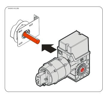
Tighten all connection elements on the drive (M8) to 25 Nm. Install all other connection elements according to the specifications of the door manufacturer.
